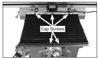
Figure 12. Front way cover installed.
